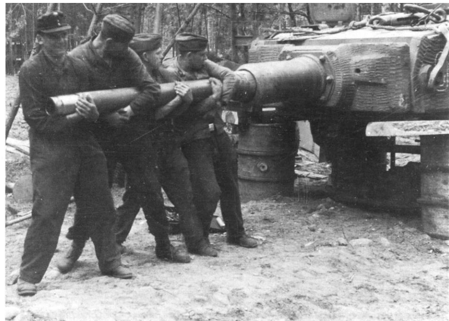
Pulling the barrel and breech of the 88mm KwK36 main gun into position required the efforts of most of the crew. The shiny threaded area on the end of the barrel is for attaching the muzzle brake to the gun tube. Timber sections are used to support the turret on the oil drums to prevent damage to the turret ring and gears.
