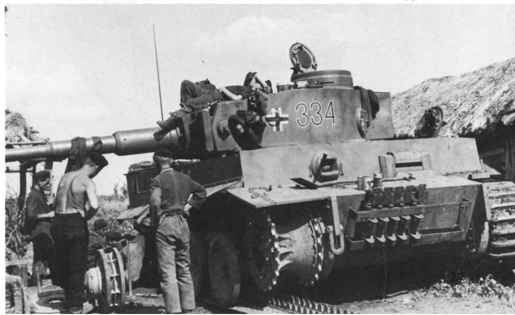
The crewmen of this Tiger of sPzAbt 503 are replacing the rear idler wheel. Although of a different style, the turret numbers on this Tiger are also in Black outlined in White. This is a replacement vehicle with new numbers, which accounts for the difference in appearance.
