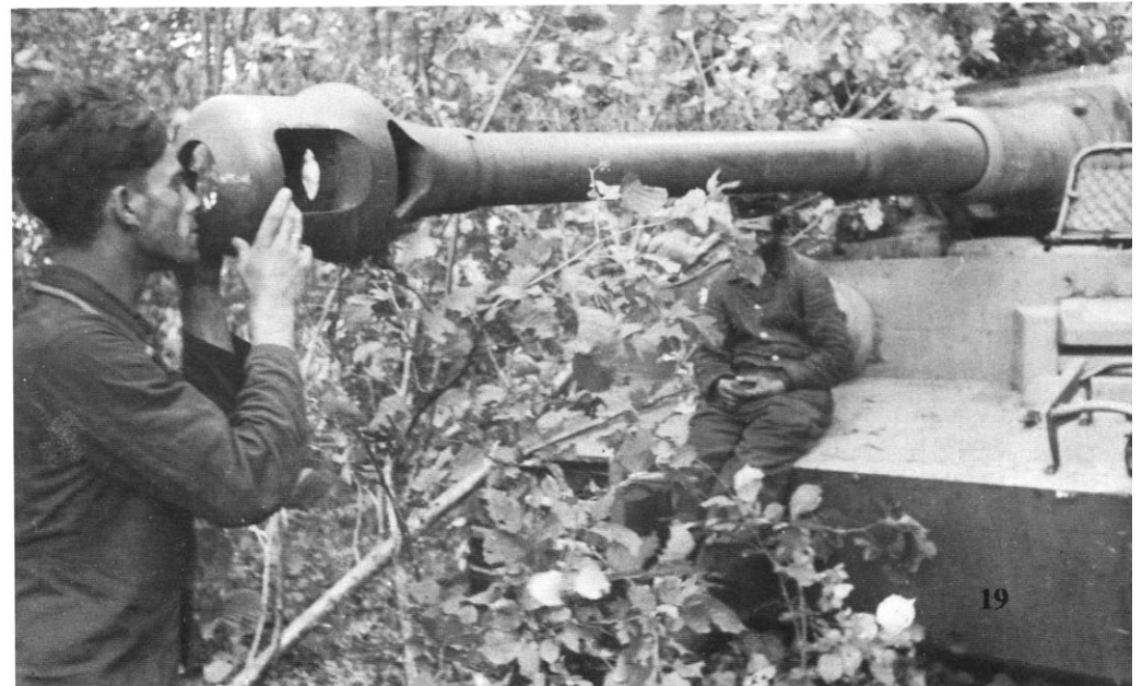
A Tiger crewman visually inspects the barrel of the main gun. After cleaning, the bore was checked for cleanliness and damage by shining a bright light into the chamber and down the barrel. This made it much easier to see the bore clearly and spot any problem areas.
