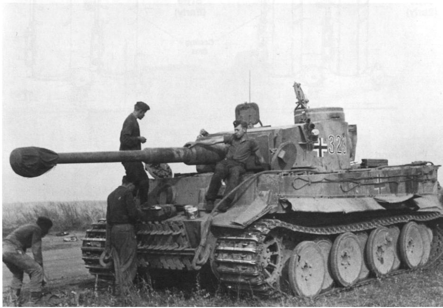
This Tiger of sPzAbt 503 reveals the kind of damage commonly suffered by the mudguards and skirts during normal combat operations. The vehicle's armor carries scars from anti-tank rifle and armor piercing bullet strikes, and the roadwheels have shrapnel damage. The turret numbers are Black outlined with White.
