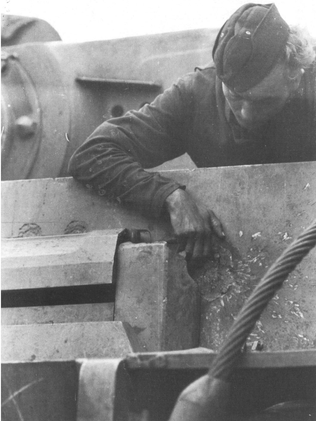
One of the reasons Tiger crews had such confidence in their vehicles was the Tiger's ability to absorb punishment. This Tiger driver examines a direct hit on his visor shield. The force of the hit has sprung the upper visor segment; however, the driver was uninjured. Most Allied tank guns could not penetrate its front armor at ranges beyond the killing range of the Tiger's main gun.
