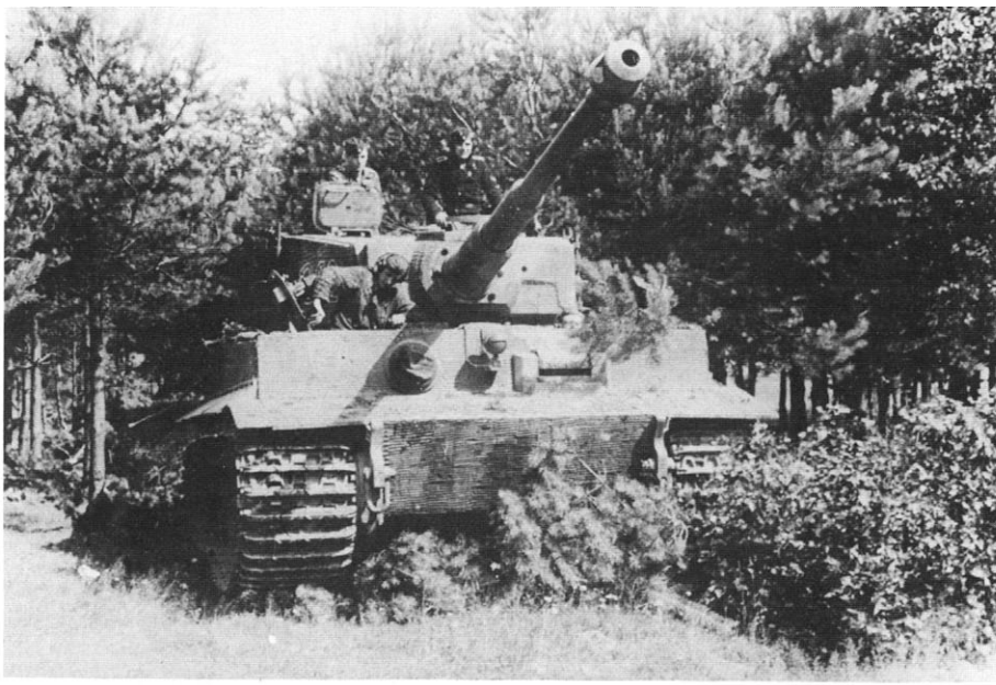
This late production Tiger ausf E reveals the major changes found on vehicles produced after February of 1944. The gunner's sight has been changed to a monocular sight, requiring only one hole in the mantlet and the roadwheels are the later steel rimmed resilient type also used on the Tiger II and on a short production run of Panther ausf Gs.
