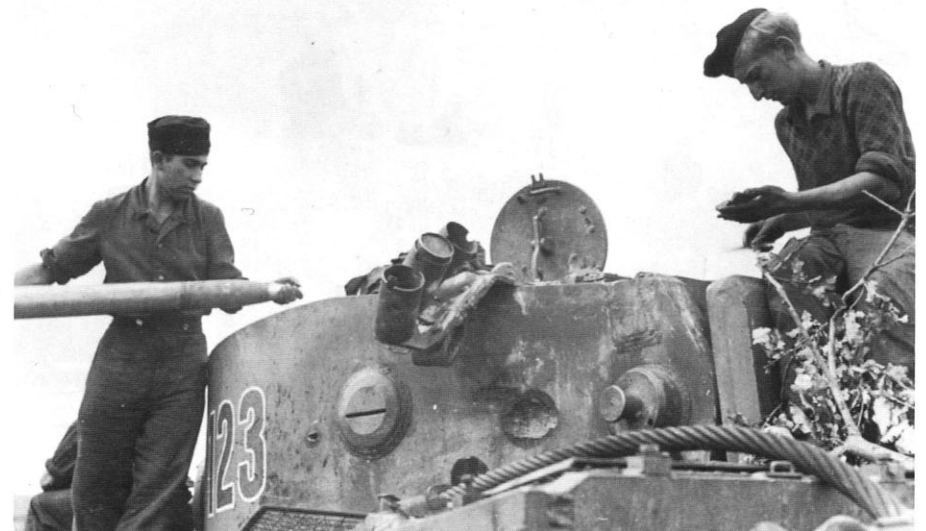
sPzAbt 503 received its first Tigers during late 1942 which were delivered in overall Dark Gray. This Tiger of the 2nd company is being overhauled in the Rostov area during early 1943 and has a PzKpfw III stowage bin fitted to the turret rear. Most Tiger units on the Russian front were forced to maintain their vehicles under very poor conditions.
