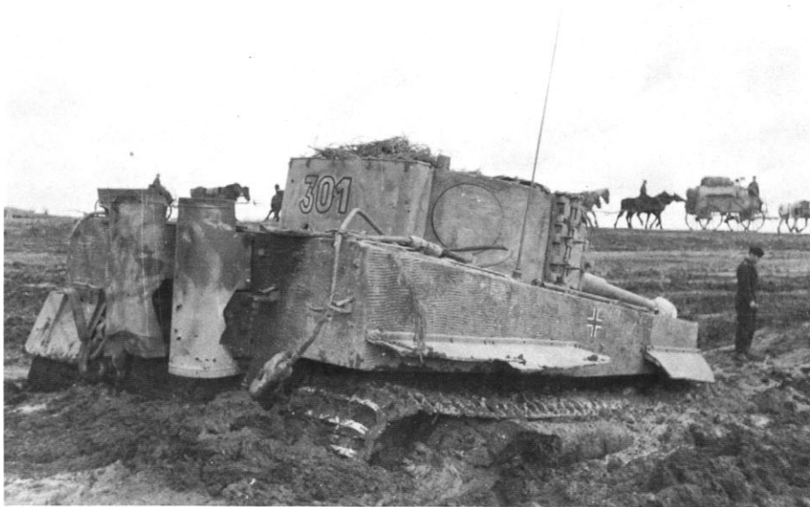
In very soft ground or mud, Tigers were prone to digging in up to the mudguards. This vehicle was eventually pulled out of the mud, but only after a great effort. The tank is painted in Dark Yellow with a light mottle of Olive Green, with the upper heat shields are in Red Brown.
