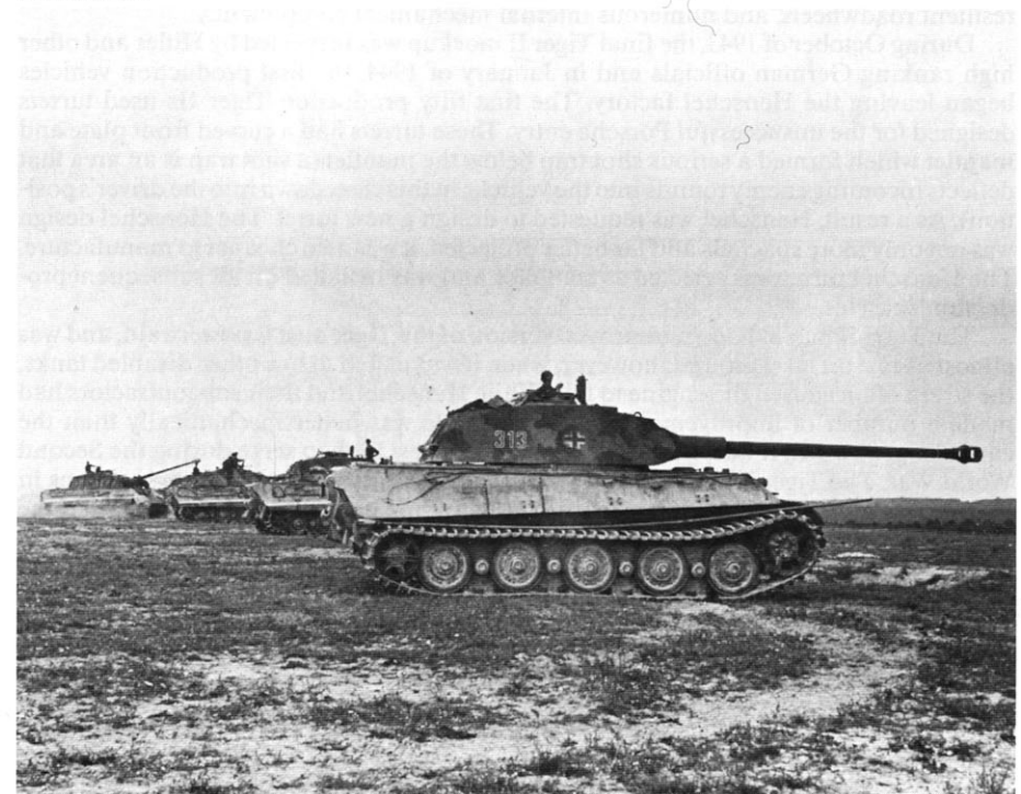
The long barrel of the 88MM L/71 KwK43 gun of the Tiger II ausf B overhung the front of the hull by a considerable distance and drivers had to exercise care when maneuvering their tanks to avoid digging the muzzle into the ground or hitting obstructions while turning the vehicle.
