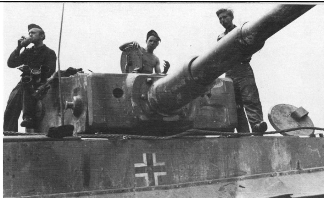
This Tiger (123) of sPzAbt 503 during the Summer of 1943 reveals the strengthened mantlet and the thickened reinforcing bar around the gunner's sight holes. This modification was introduced on the Tiger production line as a result of lessons learned during combat.
