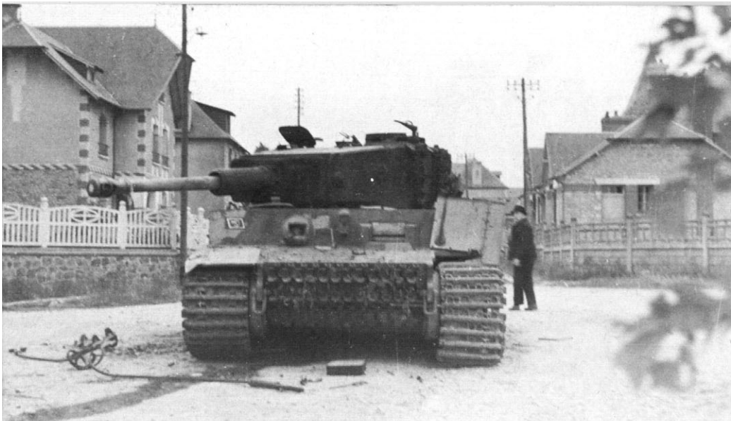
This burned out Tiger of the 1st company of SSsPzAbt 101 was destroyed in Villers-Bocage, France, on 13 June 1944. The White rhomboid marking of the 1st Company is about all that remains of the tanks original markings. The vehicle suffered an internal explosion, blowing the cupola hatch off the turret.
