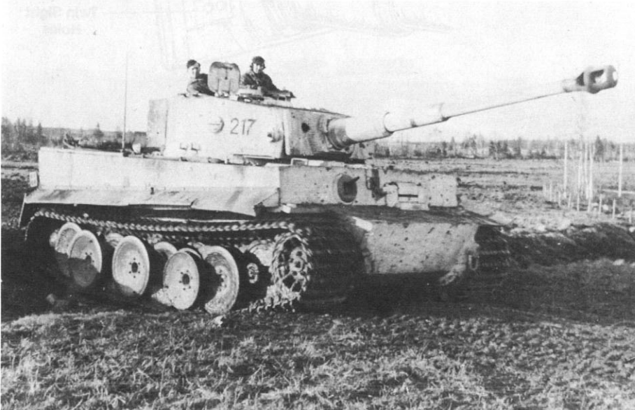
A mid-production Tiger ausf E of sPzAbt 502 crosses a ditch in the Kurland sector of the northern Russian Front during early 1945. This Whitewashed vehicle has Red turret numbers. This Tiger has the first set of roadwheels removed and also has the first outer wheel damaged.
