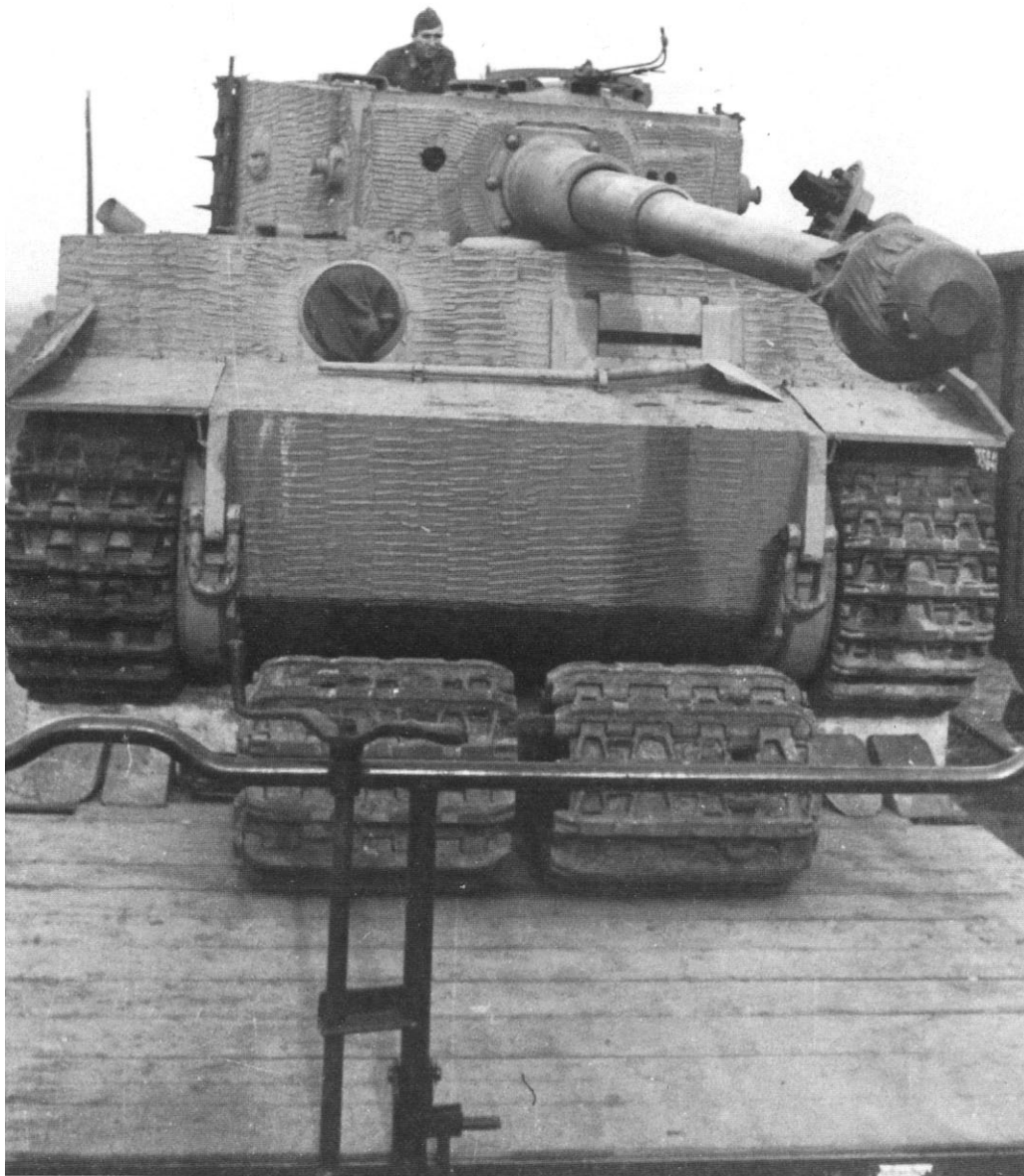
This Tiger is chained down and has the tracks blocked, ready for rail shipment to the front. It is fitted with the narrow transport tracks, with the battle tracks stowed under the vehicle. Because of the wear and tear on tank engines when they were driven long distances, most long distance tank transport was done either by rail or heavy trailer.
