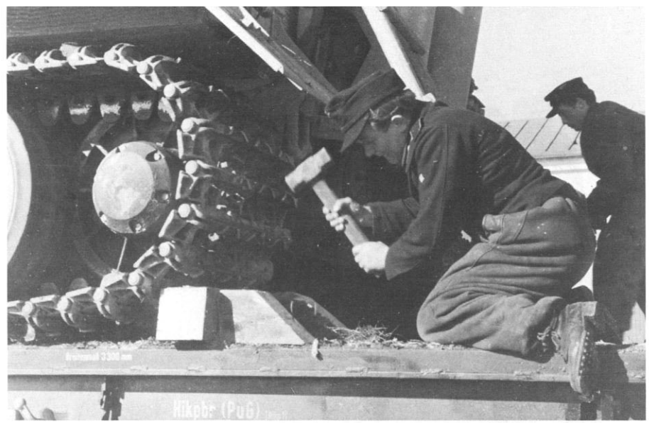
Transporting Tigers by rail usually involved removing the wide battle tracks and installing the narrower transport tracks. This Tiger, however, has been put onto a flatcar with the battle tracks installed. Although the narrow clearances in Germany and Europe led to the use of narrow transport tracks, in Eastern Europe and in rural areas the railroads were often open enough to allow the battle tracks to be left on.
