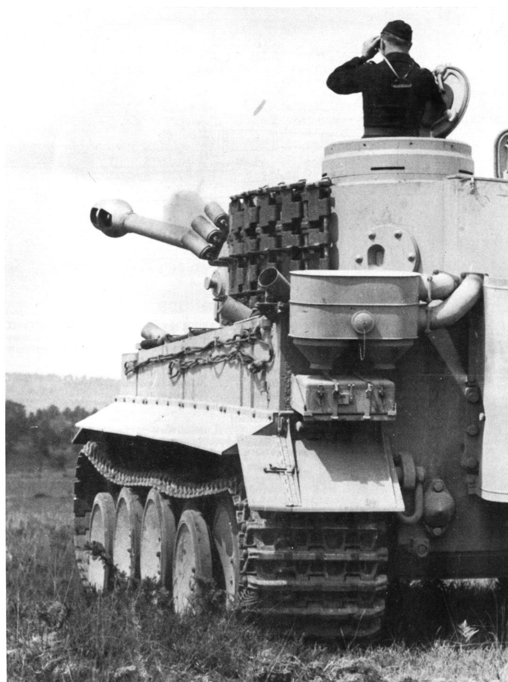
The Feifel air filters were mounted on both the port and starboard sides of the rear engine deck above the mud flaps. The three short tubes on the hull top are "S" anti-personnel mine dischargers. The Feifel air cleaners were prone to damage after short periods of service and were often removed. They were, however, effective in preventing premature wear and damage to the engine from dust.
