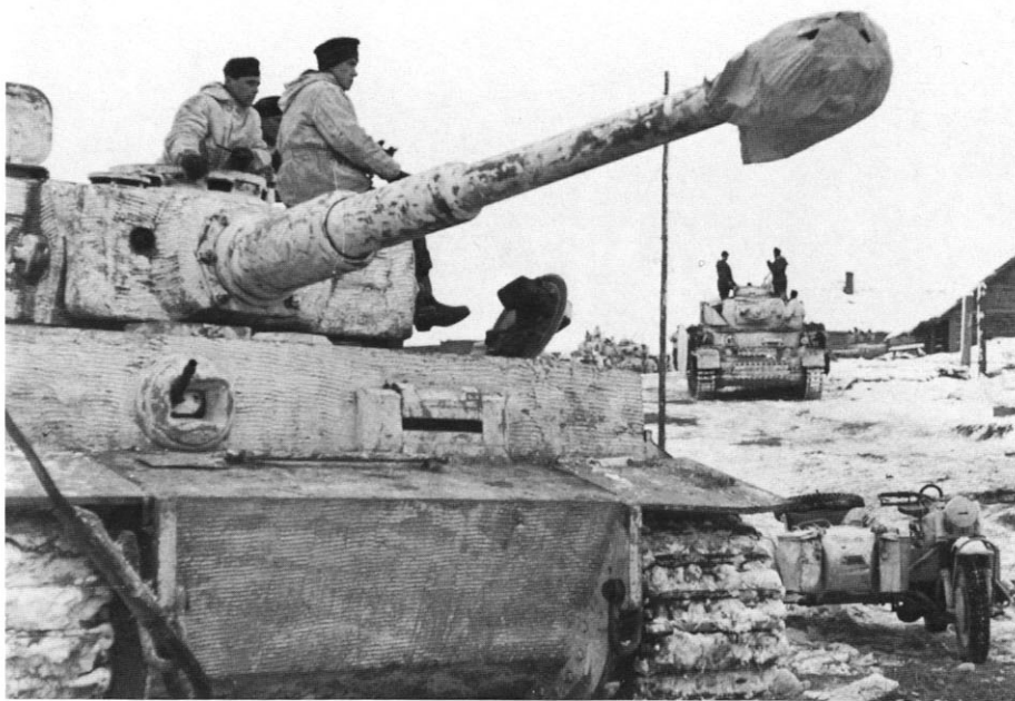
Tigers, along with many other German tanks, were coated with zimmerit anti-magnetic cement applied to the vertical surfaces as protection from magnetic mines. Normally the zimmerit coating for the Tiger was applied at the factory with a toothed trowel or blade which produced a characteristic rough texture.
