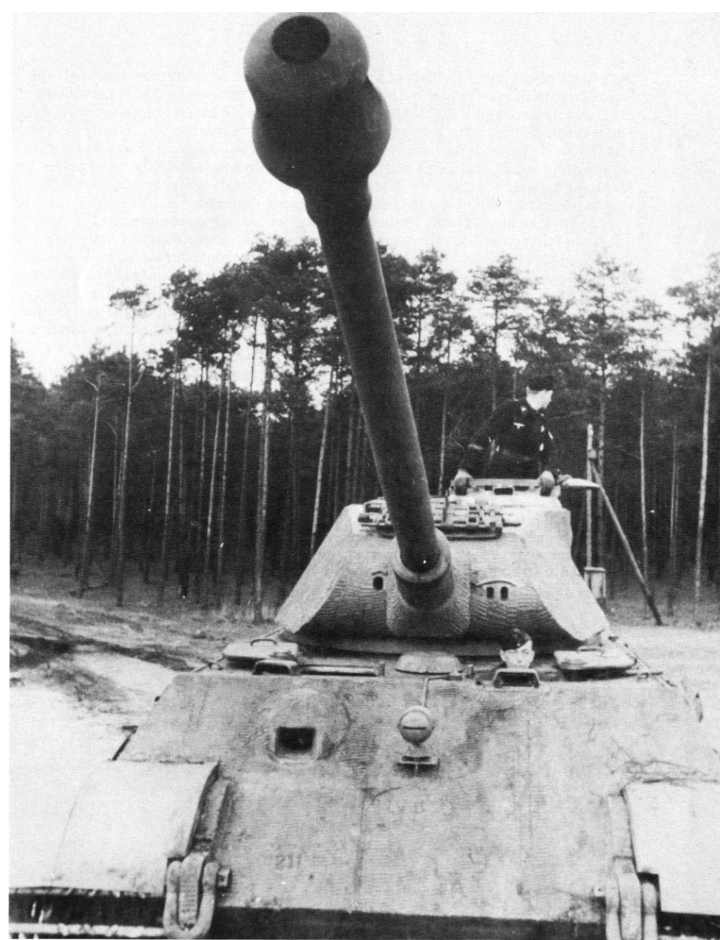
This early Tiger II ausf B is fitted with the Porsche designed turret which used a binocular gunner's sight. The curved front plate created a serious shot trap which deflected incoming rounds down into the driver's compartment. The bulge for the cupola also was a weak area in the turret side armor. The production Henschel turret eliminated these deficiencies.
