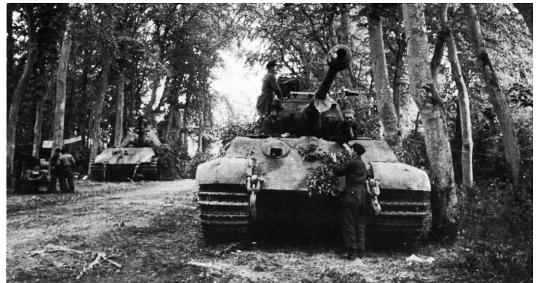
Tiger II ausf Bs of the 1st company of sPzAbt 503 in Normandy are parked under the trees and have foliage applied to them in order to hide them from Allied aircraft. The Tiger II in the foreground has all the side skirts fitted; however, the Tiger II in the background has no skirts fitted.
