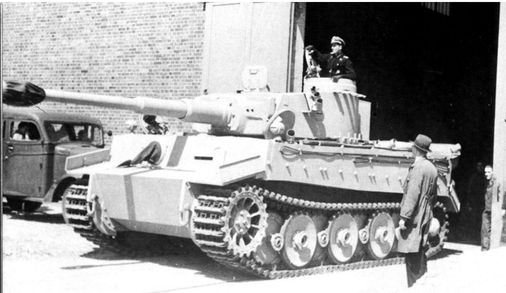
A new production Tiger leaves the final assembly building at the Henschel plant. This is a mid-production vehicle; however, it retains many of the main features of early Tigers. The small angled tubes mounted on the hull top are "S" anti-personnel mine dischargers.
