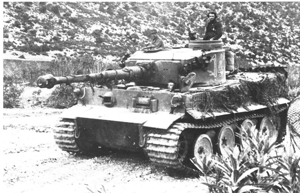
Tiger 142 of sPzAbt 501 advances down a road in Tunisia. The Tiger has the unit field modifications, the lowered headlights and modified mudguards, that made the tanks assigned to sPzAbt 501 unique. The tank is camouflaged in overall Brown, possibly with an over spray of Olive Green. The turret number is Red outlined in White outline.
