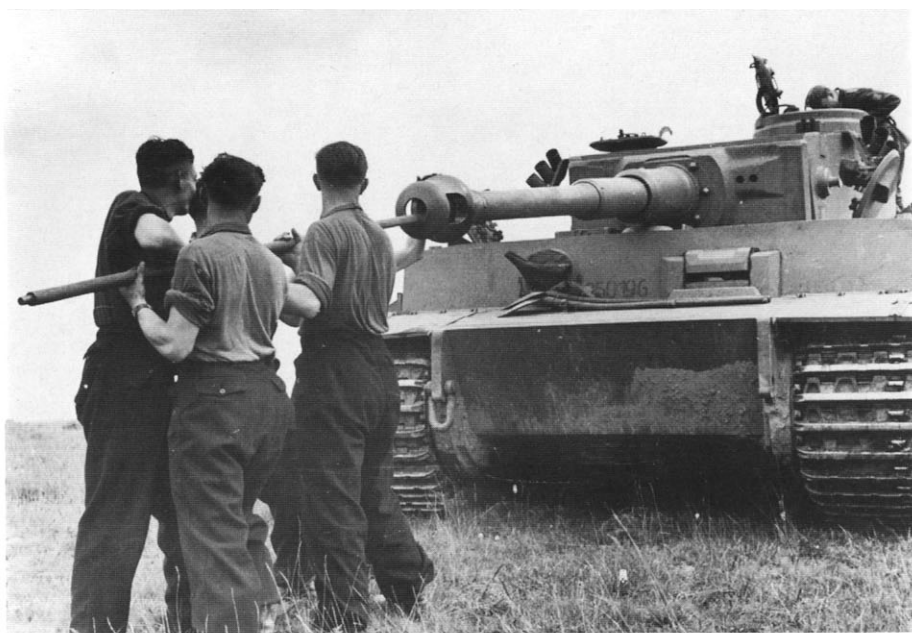
The crew of this Tiger cleans out the barrel of the 88mm KwK36 main gun. Two or three men were required to swab out the bore, and one crewman remained in the turret to clean out the chamber and check the bore. This Tiger of sPzAbt 502 was later destroyed during August of 1944 by a Russian 85mm anti-tank gun.
