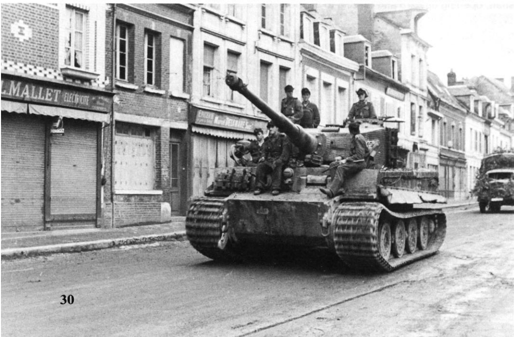
This late production Tiger ausf E of sPzAbt 503, advancing through a French town in Normandy during August of 1944, reveals the new roadwheels and monocular gunner's sight. With the new road wheel design, the outer row of wheels, normally removed during rail transport, have been eliminated entirely. This Tiger is Dark Yellow with heavy mottling of Olive Green and Red Brown with the turret numbers in Black with White outlines.
