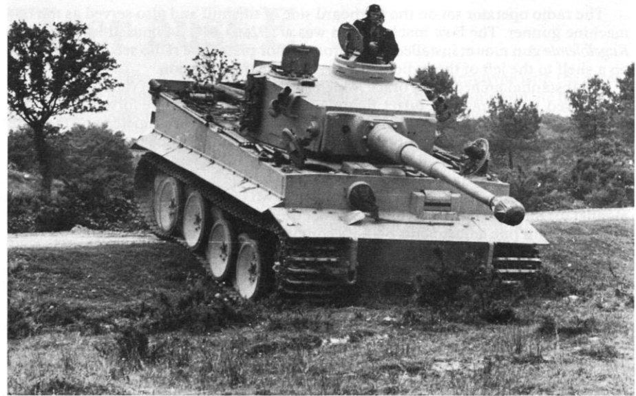
This new production Tiger crosses a road during unit training exercises held in early 1943. It usually did not take long for the skirts and mudguards to begin to show signs of damage caused by running through brush and trees. Often, even heavier external parts were damaged by repeated heavy use and maintenance.
