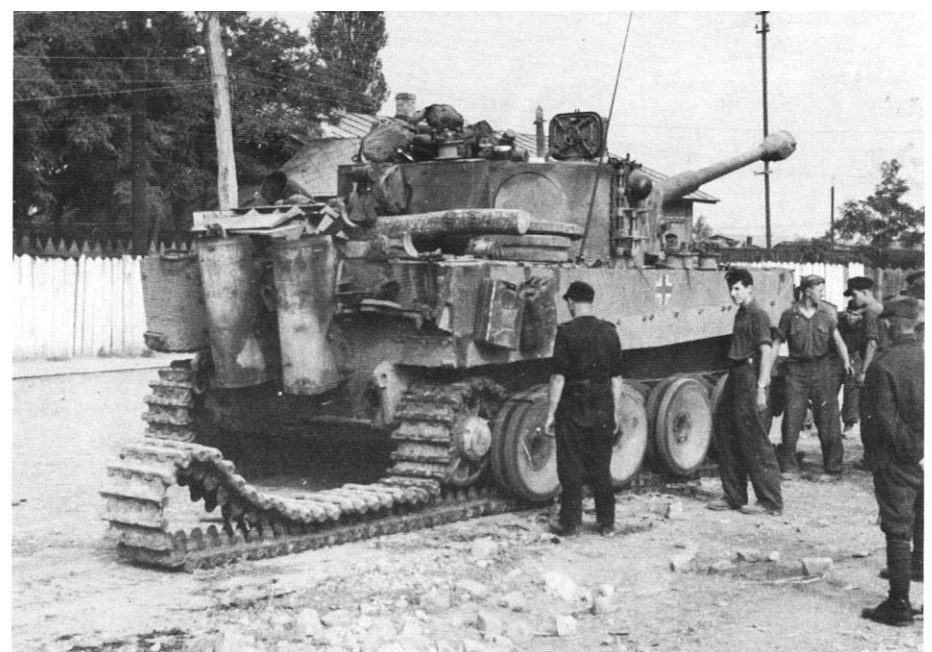
This Tiger of Grossdeutschland is being prepared for rail transport. The cable attached to the narrow transport track leads up to the drive sprocket which will pull the track up to the front of the tank where the crew will join the two ends. This Tiger is Dark Yellow with Red Brown patches and light Olive Green mottling with the turret number, A32, in Black.
