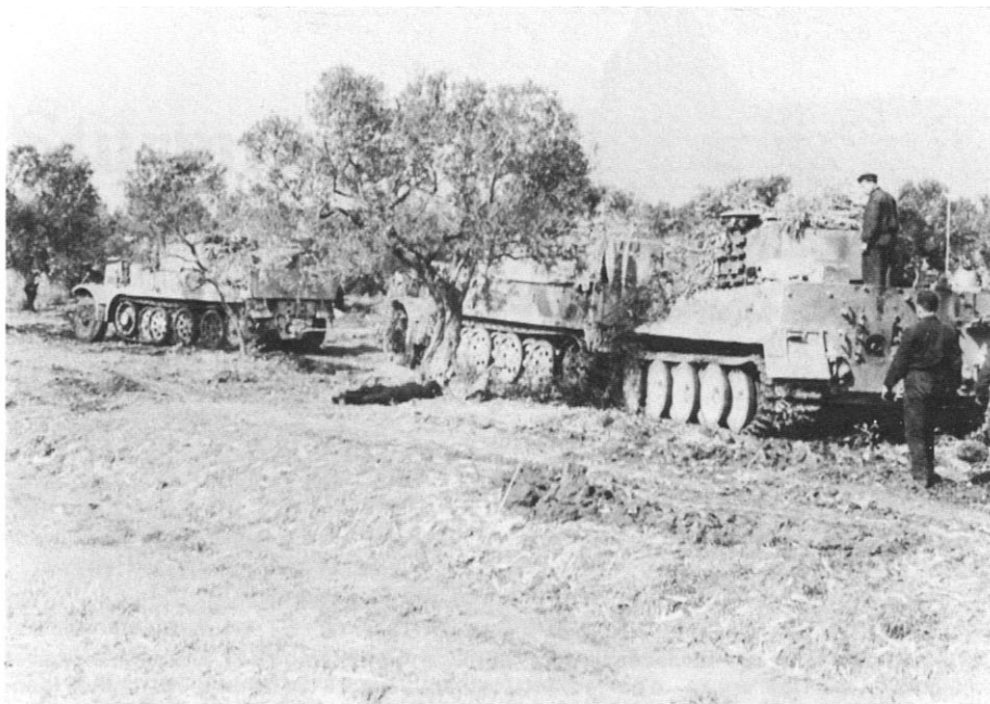
Two eighteen ton SdKfz 9 tractors tow a disabled Tiger of sPzAbt 508 into a grove of trees for repairs. Between 23 and 25 May 1944, the 3rd company of sPzAbt 508 lost fifteen out of its sixteen Tigers, most to mechanical breakdowns. The lack of heavy recovery vehicles cost German units a number of vehicles they could have otherwise retrieved.
