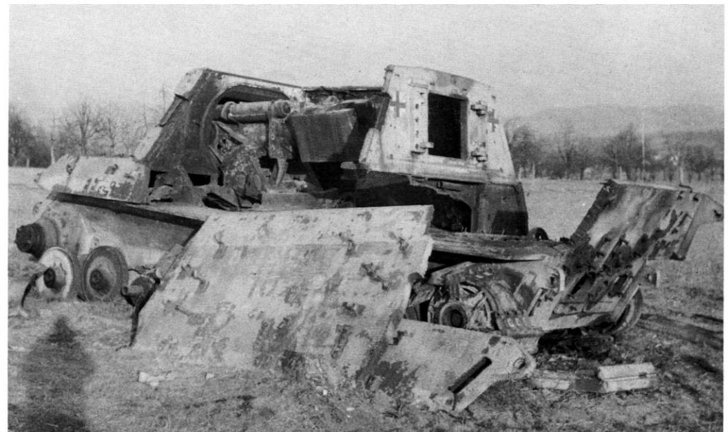
One of the two experimental Jagdtigers , which were fitted with the Porsche suspension system, was issued to sPzJagAbt 653 and was later destroyed by its crew. The tremendous force of the demolition charge placed inside the vehicle has torn apart the superstructure, blown off the gun barrel, and thrown the engine completely away from the vehicle.
