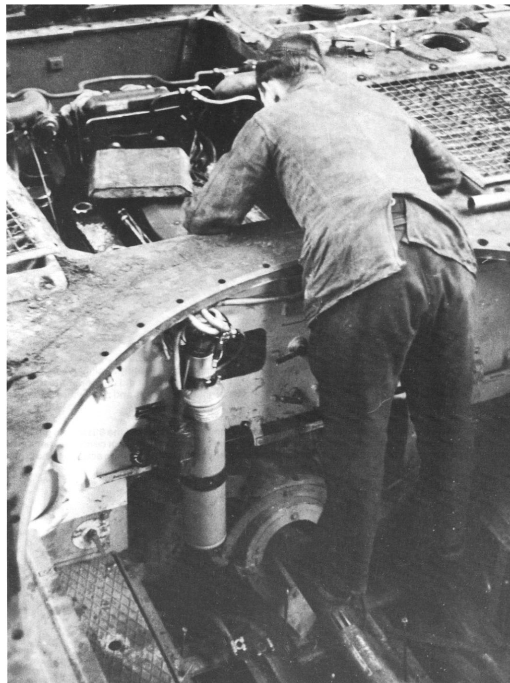
The crew of this Tiger has raised the rear engine cover to gain access to the engine compartment. Normally, repairs were made in rear areas and under cover to protect the immobile Tiger from detection and destruction by enemy aircraft.
