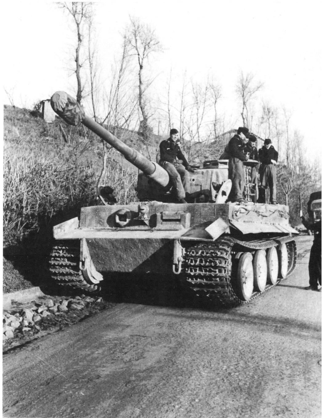
This Tiger of sPzAbt 508 is Dark Yellow over sprayed with Olive Green and Red Brown. The vehicle has had the bow MG 34 machine gun removed, indicating that it is well behind the lines, traveling to a unit organization point. Although rail transport was preferable, tanks were driven fairly long distances when rail travel was not possible.
