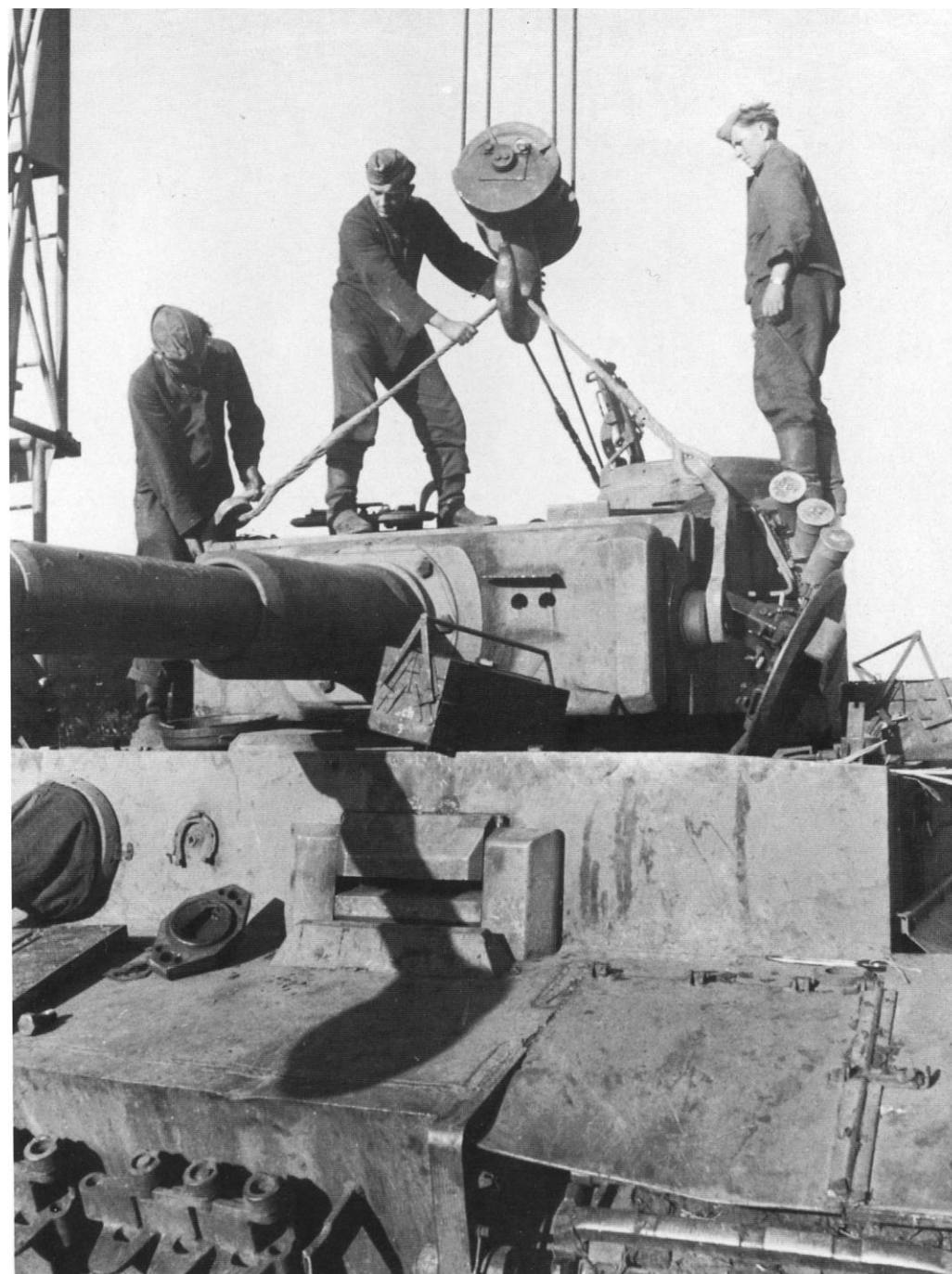
Any major work that had to be done on the transmission or final drive usually required the removal of the turret. Repair crews position lift hooks and cables from an overhead gantry crane to the lift points on the Tiger's turret prior to lifting the turret off the hull.
