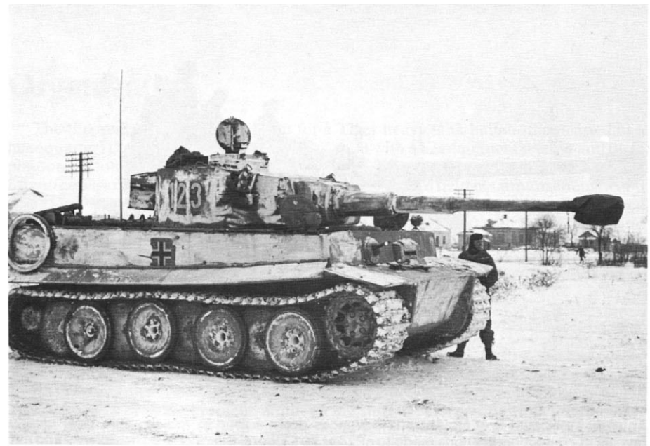
This Tiger of sPzAbt 503 is overall Dark Gray with a coat of White winter camouflage paint applied directly over the original camouflage. The winter camouflage paints were scarce and were applied in the field resulting in a very rough appearance. The turret numbers are White with a thin Black outline. This Tiger also carries a PzKpfw III stowage bin.
