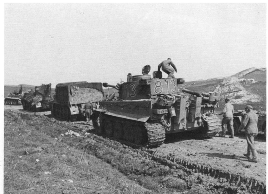
This Tiger of sPzAbt 501, was attached to PzRgt 7, 10.PzDiv, and has large Red and White turret numbers applied over an overall Brown camouflage. This vehicle is fitted with early style square heat shields on the rear exhaust manifolds and stacks. These shields were later changed to a rounded style with cooling vents.
