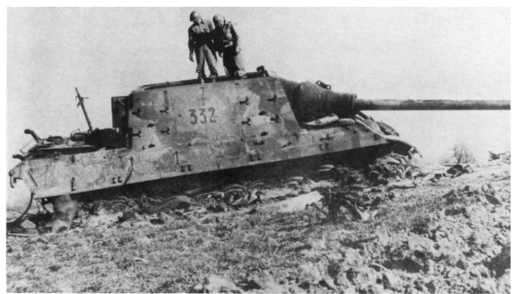
A Jagdtiger of the 3rd company of JgTgrAbt 512, is examined by U.S. troops after it was blown up by its crew. The whole top turret roof plate is gone and the 128MM PaK44 main gun has been blown out of its mount. The colors are Dark Yellow with Red Brown over a base of Dark Gray. The side number, 332, is Black with a White outline. (U.S. Army)
