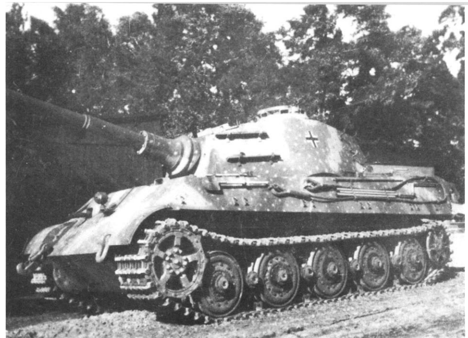
The late war ambush dappled camouflage paint scheme was not used on Tiger IIs often. As these heavy tanks began being used in defensive positions, such patterns became more widely used. The dappled spots are Dark Yellow over the standard three-color camouflage scheme. This vehicle also still has its narrow transport tracks fitted. (Eric Helmuth)
