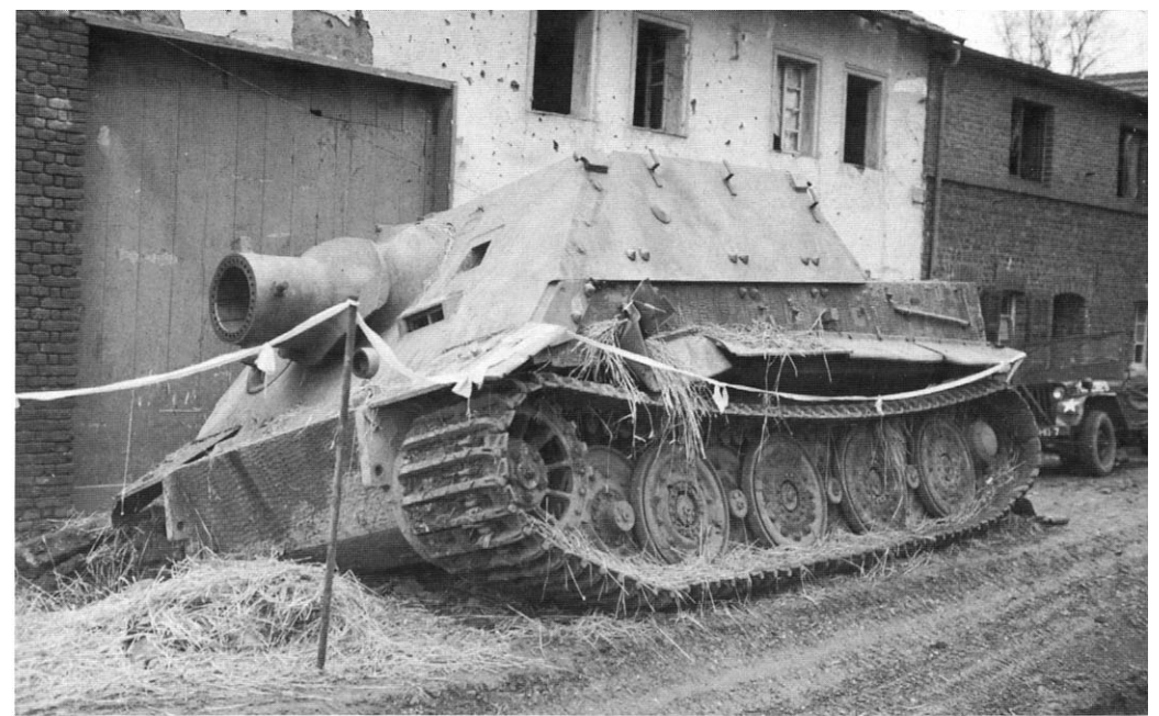
The only major variant of the Tiger ausf E to reach production was the Sturmtiger built on a late Tiger chassis with resilient steel rimmed roadwheels. With 150MM of front armor, the Sturmtiger was virtually impossible to penetrate with any Allied tank ammunition. The vehicle was intended to destroy fortified positions and buildings with its huge weapon. (U.S. Army)
