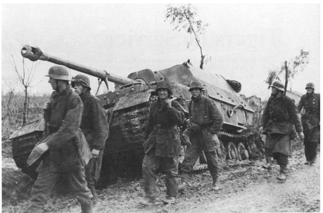
This Elefant of PzJagAbt 653 suffered the fate of most of these vehicles in Italy. Designed for open long-range anti-tank engagements, the vehicles were ill-suited for the hilly terrain and muddy conditions found on the Italian front. Many disabled vehicles were towed to fixed positions where their 88mm guns could command a critical road or other military objective.
