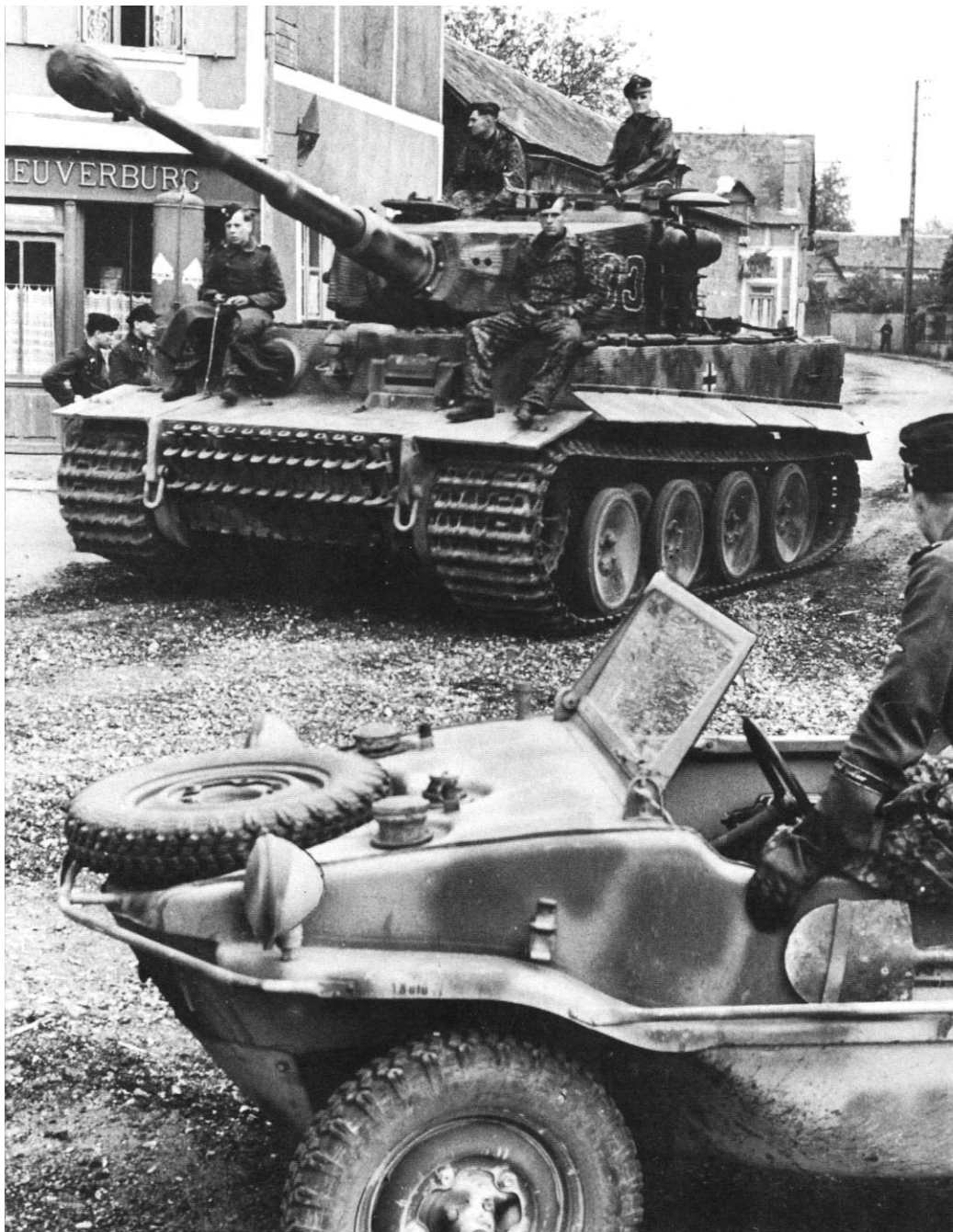
A Tiger of the 1st company, SSsPzAbt 101 drives through a French village past a Schwimmwagen amphibious car during 1944. Tigers of 1st Company used White outlines on the turret numbers (if the number was painted on a dark area of the turret). Tiger 133 reveals this practice with White outline numbers against the dark camouflage on the turret side. The outlines were often filled in with brushed paint or masked off during spraying.
