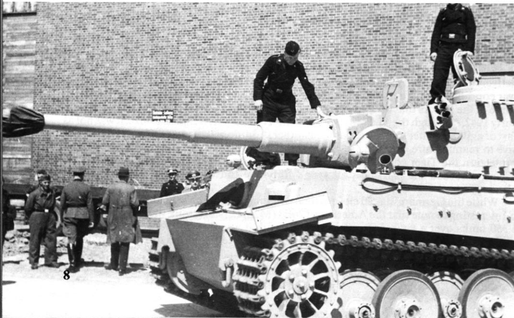
The bolts on the hull sides are used to attach the side skirts. The narrow transport tracks were required to avoid excess overhang during rail shipment of Tigers to the front. Many tunnels and bridges were too narrow to allow a fully tracked Tiger to clear, especially on curves.
