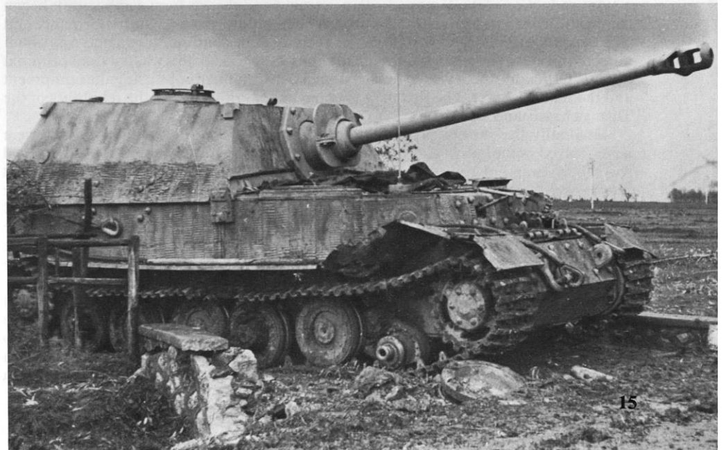
This abandoned Elefant was put out of action when a mine damaged its suspension. Often the loss of a roadwheel resulted in the loss of the vehicle. This Elefant is camouflaged in Dark Yellow with a mottle of Olive Green and Red Brown and has a coating of zimmerit anti-magnetic mine paste on the lower sides.
