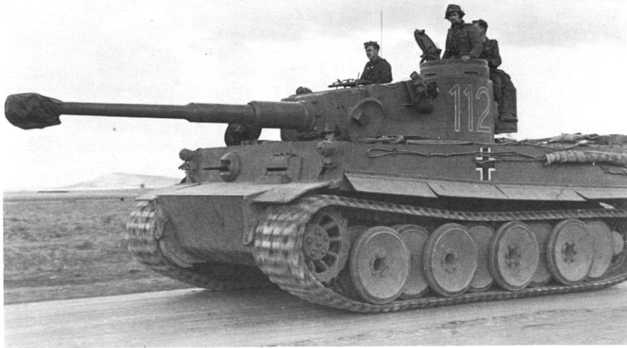
An early Tiger ausf E of sPzAbt 501 advances down a road in Tunisia. This Tiger clearly reveals the field modifications made to sPzAbt 501 Tigers, the relocated headlights and cut down fenders.
