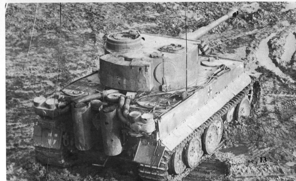
Tiger 131 was displayed by the British in Tunisia after being repainted for an inspection by King George VI. The shield on the mudguard is from the British First Army which captured this vehicle. The large round loading hatch on the turret rear replaced the second pistol port found on early production Tigers.
